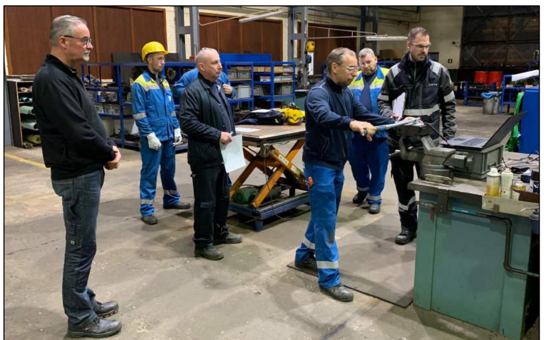
Hand torqueing with 100. [Nm] at calibration device.
