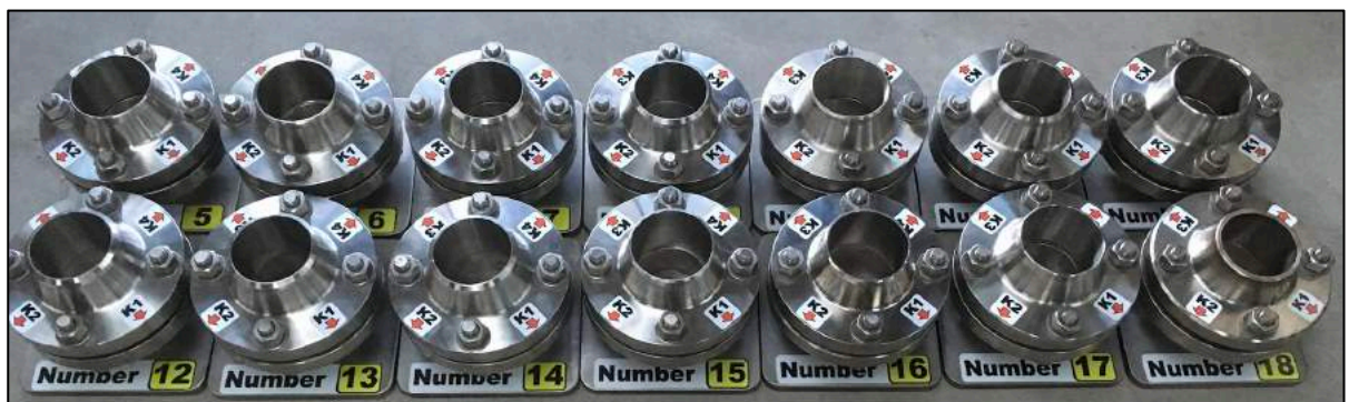
3" 150# flange assemblies to test the competency of measuring the flange gaps
