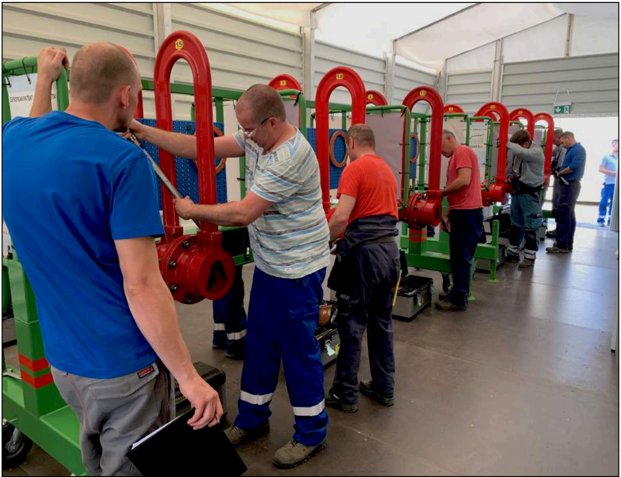
Break-loose measurements by assessor using an electronic hand torque wrench
