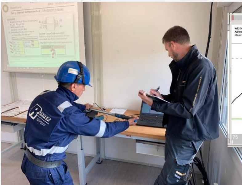
Hand torqueing with 100. [Nm] at calibration device.
